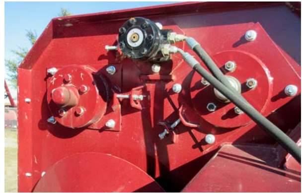
FIG. 101 BAG ROLLER CHAIN DRIVE TENSION
